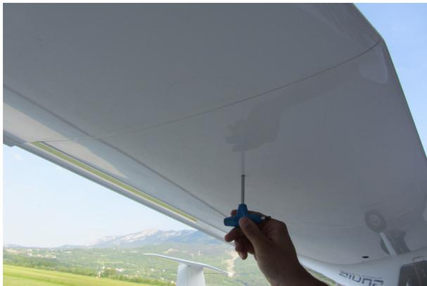
Insert the provided key into the BOTTOM service opening on the main wing and screw the bolt into position. Make sure the bolt is tight, verify the bolt's fit also by checking that the bolt-end aligned itself with the surface of the wing at the top service opening
