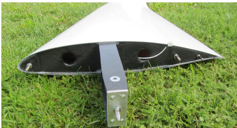
The procedure to install the optional removable wingtips begins by cleaning both the front and aft bushing and pin on the wing and the wingtip.
