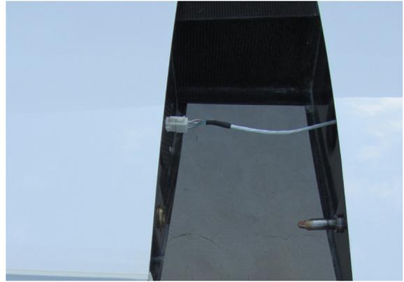
Connect the wingtip lights cable if equipped with the connector provided. Push the wingtip into position, making sure the gap between the wing and the wingtip is equal all along and the wingtip is not inserted at an angle.
